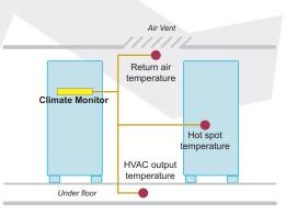
Remote temperature sensors attached to this climate monitor to provide temperature values for critical areas.
